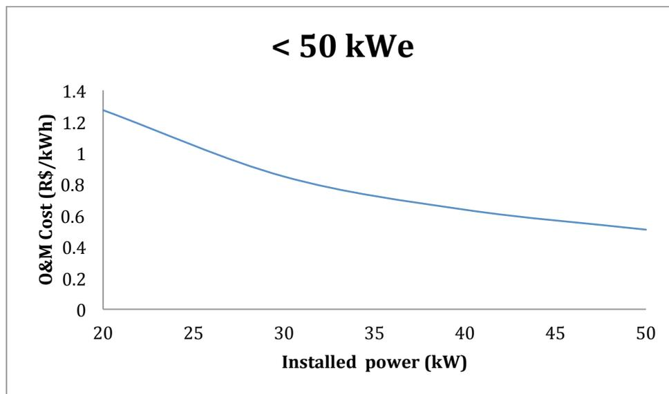
Figure 21: Operation & Maintenance costs for plants for electric power generation below 50 kW. Source: (Santos, 2007)
