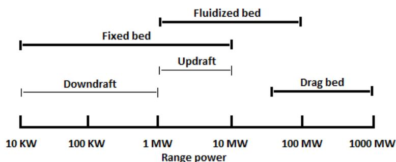
Figure 23: Gasifier in the power range. Source: elaborated by the authors based on Kinto (2012)
