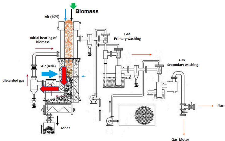
Figure 25: Biomass (downdraft gasifier). Source: Adapted from Gaseifamaz (CENBIO, 2006).
