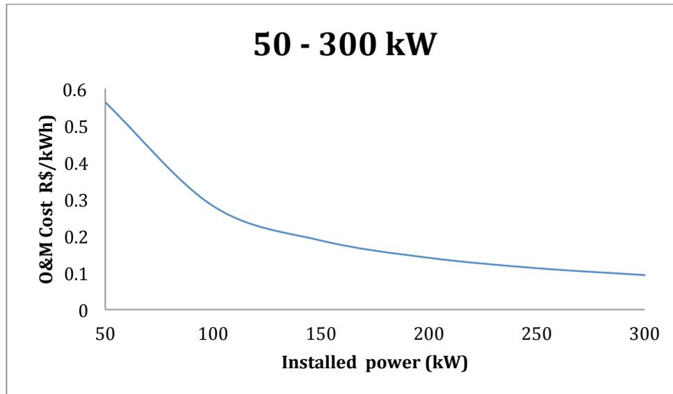
Figure 22: Operation & Maintenance costs for plants for electric power generation between 50-300 kW.
