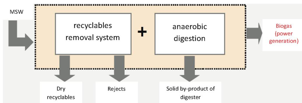
Figure 35: Anaerobic digestion of MSW through biodigester Source: Adapted from (ARCHER, 2005)
