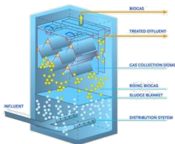
Figure 31: UASB Biodigester. Source: (PAQUES, 2013).
