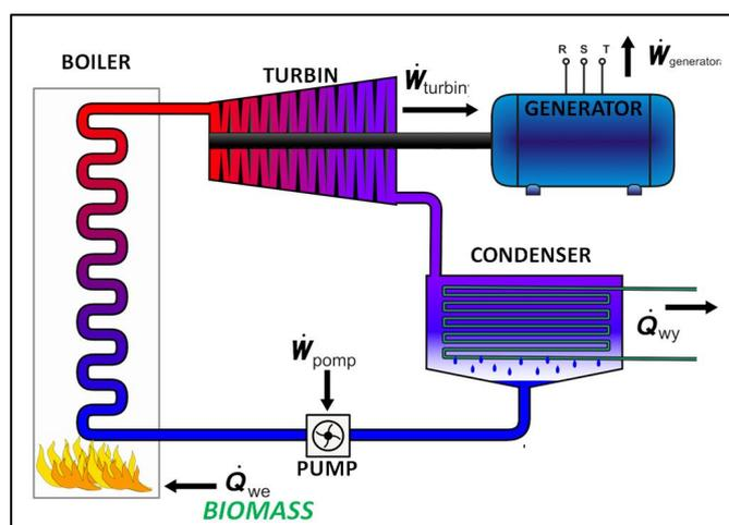
Figure 18: Simple Rankine cycle. Adapted from (Ainsworth, 2007)
