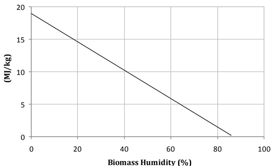
Figure 27: Heating value of wood due to its humidity. Source: Elaborated by the authors
