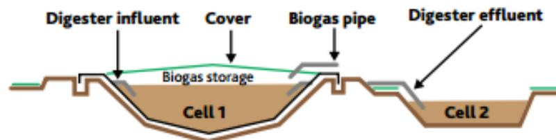
Figure 33: Covered lagoon schematic<sup>33</sup>
