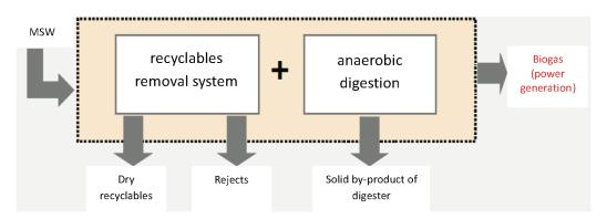
Figure 35: Anaerobic digestion of MSW through biodigester Source: Adapted from (ARCHER, 2005)
