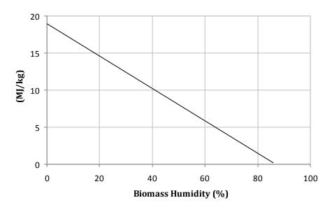
Figure 27: Heating value of wood due to its humidity. Source: Elaborated by the authors
