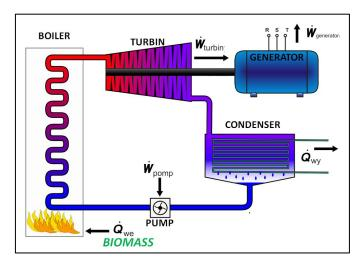
Figure 18: Simple Rankine cycle. Adapted from (Ainsworth, 2007)
