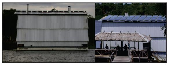
Figure 20: Mobile power unit project hybridized with PV panels. Source: (Nogueira, 2012)
