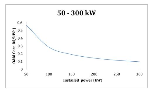
Figure 22: Operation & Maintenance costs for plants for electric power generation between 50-300 kW. Source: (Santos, 2007)
