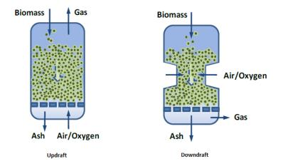
Figure 24: Types of Fixed bed gasifiers. Source: Adapted from E4 Tech (2009)
