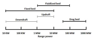
Figure 23: Gasifier in the power range. Source: elaborated by the authors based on Kinto (2012)
