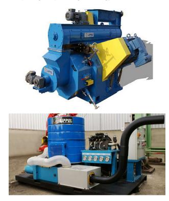
Figure 29: Briquetting and pelletizing technology in small-scale. Source: Lippe
