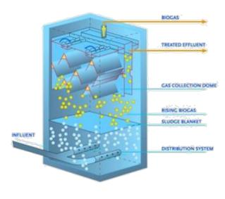
Figure 31: UASB Biodigester. Source: (PAQUES, 2013).
